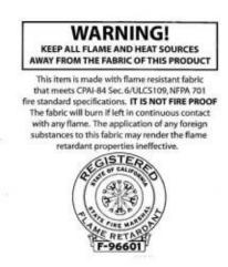
The side walls, drops, awnings and tops of booths, membrane structures, canopies, and tents shall be composed of flame-resistant material or shall be treated with an approved flame retardant. The use of non-treated polyethylene tarps and "Blue Tarps" during the hours of the public use is prohibited.
